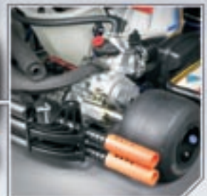
Rotax Rear Tire Protection System (RTPS)
