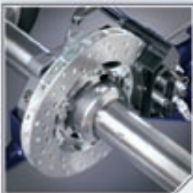
Radially vented 18mm wide rear brake disc and machined billet alloy 4-spot brake caliper mounted directly to bearing flange
